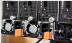
NF3 is a versatile hi-rel system that supports 2N redundancy and automatic failover. It uses four 2.2 KW hot-swap redundant power supplies delivering up to 225 Watts of independent power into each bay. Special monitoring system handles abnormal power consumption scenarios ensuring several levels of power surge protection.
