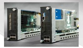
Each board sits in its own hot-swap bay. 8 in the front and 8 in the back. All are compatible with any off-the-shelf FPGA board from any manufacturer (PCle form factor: full-height, full-length and double-slot). All bays are synchronized through a common reference clock, jitter-cleaned per each bay.
