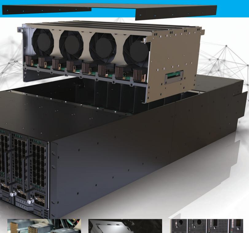
Once inserted, each bay run-time connects to the switching system through twenty 12.5 Gbps lanes. 16 go to the PCle connector, the other 4 go to the SFP+ or QSFP ports on its front panel allowing direct external access to the Layer 1 interconnect fabric. Data delivered from external port can be broadcasted to all 16 boards right away.
